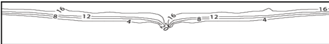
Figure 4.18: Computed tracer concentration distribution in the vertical section across the discharge point for a plane vertical “jet-like” buoyant jet in uniform ambient at selected times (contour in 0.01C_o ).
